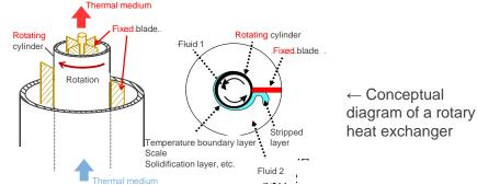
The higher the rotational speed, the better the heat transfer performance (overall heat transfer coefficient)
