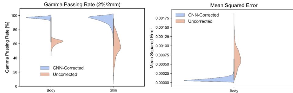
The CNN-corrected (CNN-corrected) dose distribution shows good agreement with the true value which is the dose distribution with magnetic field, compared to uncorrected one (uncorrected).
