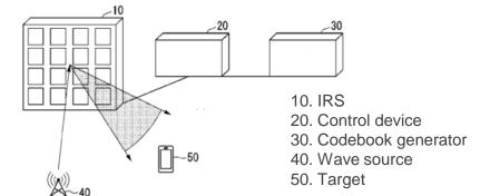
Possible to control IRS depending on reference value, and to control IRS without CSI
