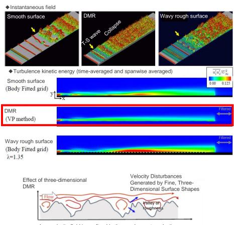
•Low velocity fluid is confined in the roughness trough, the occurrence of ejection is suppressed, and turbulent kinetic energy is suppressed.
