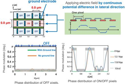
Independent driving was possible with pixel pitch of 0.8  $\mu$ m according to liquid crystal alignment simulation.
